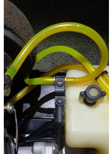
4. The remaining fuel line can now be used to connect the suction line from tank barb to carburettor (bottom barb).
