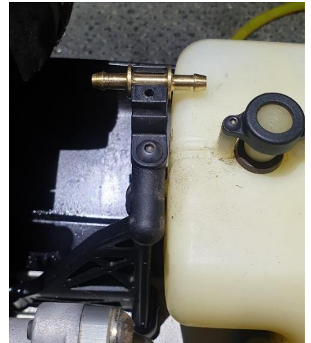
2. Install RTE Losi Fuel Line Adaptor.
