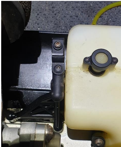
4. Remove Losi fuel line mounting, and rotate 180°
