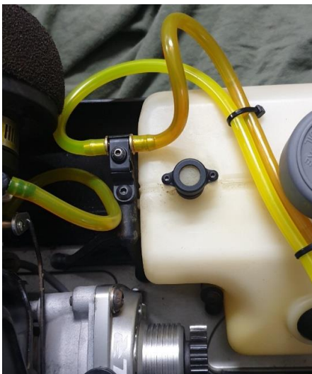
8. Connect this line from the top return line barb on the carburettor, to the Losi adaptor.
