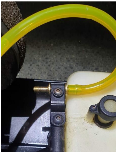
7. Cut a length of fuel line approximately 15cm (6") from the end of the return line (installed in grommet).
